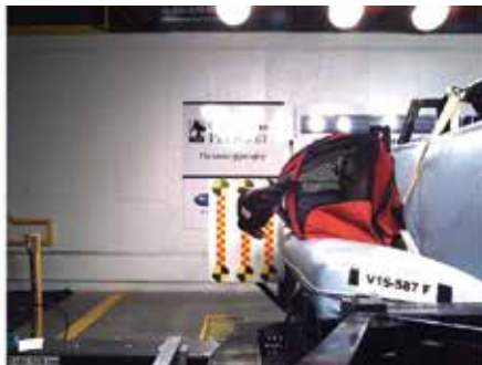
Front of carrier completely tears
