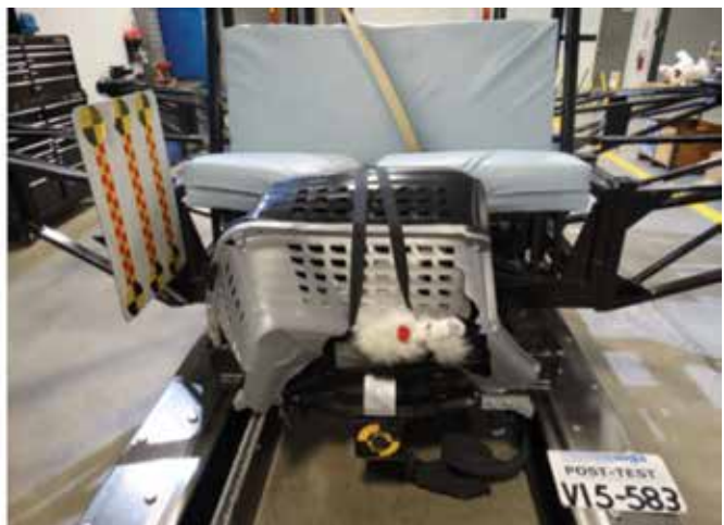
During and Post-test images of PetBuckle Restraint System securing the Carrier/Kennel
