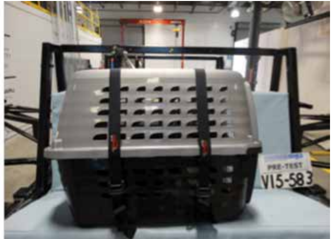
Pre-test images of PetBuckle Restraint System securing the Carrier/Kennel
