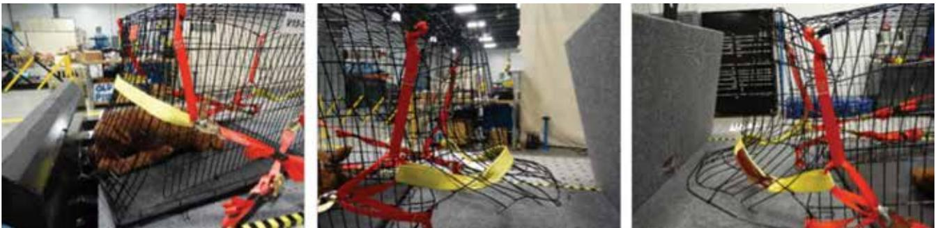
*Wire Crate w/ Reinforced Cage Support Strap System Post-Test*
