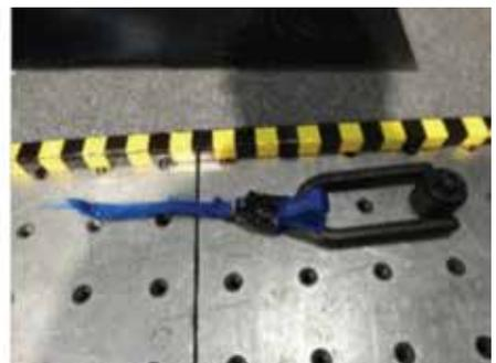
MIM Variocage Post-Test 1. Complete connection failures (Front and Rear)
