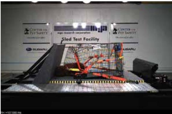
*Major crate deformation allowing partial ejection of dog*
