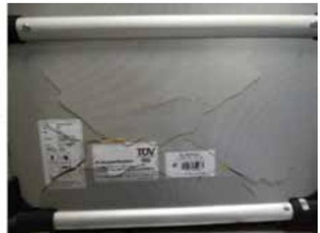
*ProLine Milan Post Test 2. Connection to seatback intact, crate door release inwards, wooden back panel damage.*
