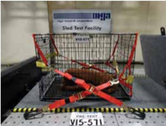
*Wire Crate w/ Reinforced Cage Support Strap System Pre-Test*
